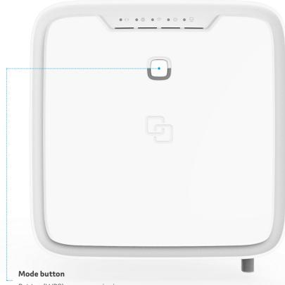
Pairing (WPS) – press and release once WiFi ON – press and hold until WiFi LED turns solid green WiFi OFF – press and hold until WiFi LED turns off
